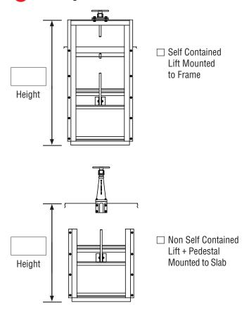
**Lift:** Manual handwheel or handcrank will be provided, based on gate dimensions furnished.
